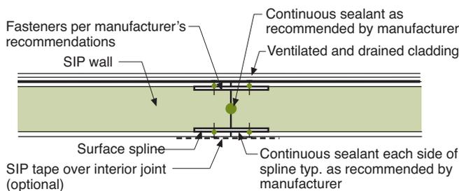
Details 1.1 through 1.7 depict different types of spline joints connecting panels (not to scale). As previously mentioned, solid lumber insulates less and transfers energy. Wood typically has an R-value of 1/inch compared to EPS foam at 3.6/inch minimum R-value as per ASTM C578 Type I foam. This is why the box/block and surface splines are more thermally efficient than solid wood. A box/block and surface spline can be thought of as an 'insulating spline.'
