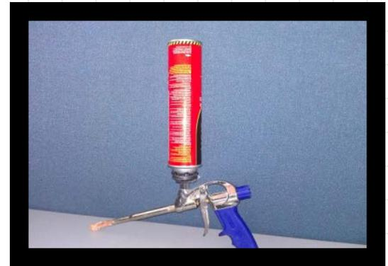
Figure 15. Spray Foam Application Gun
