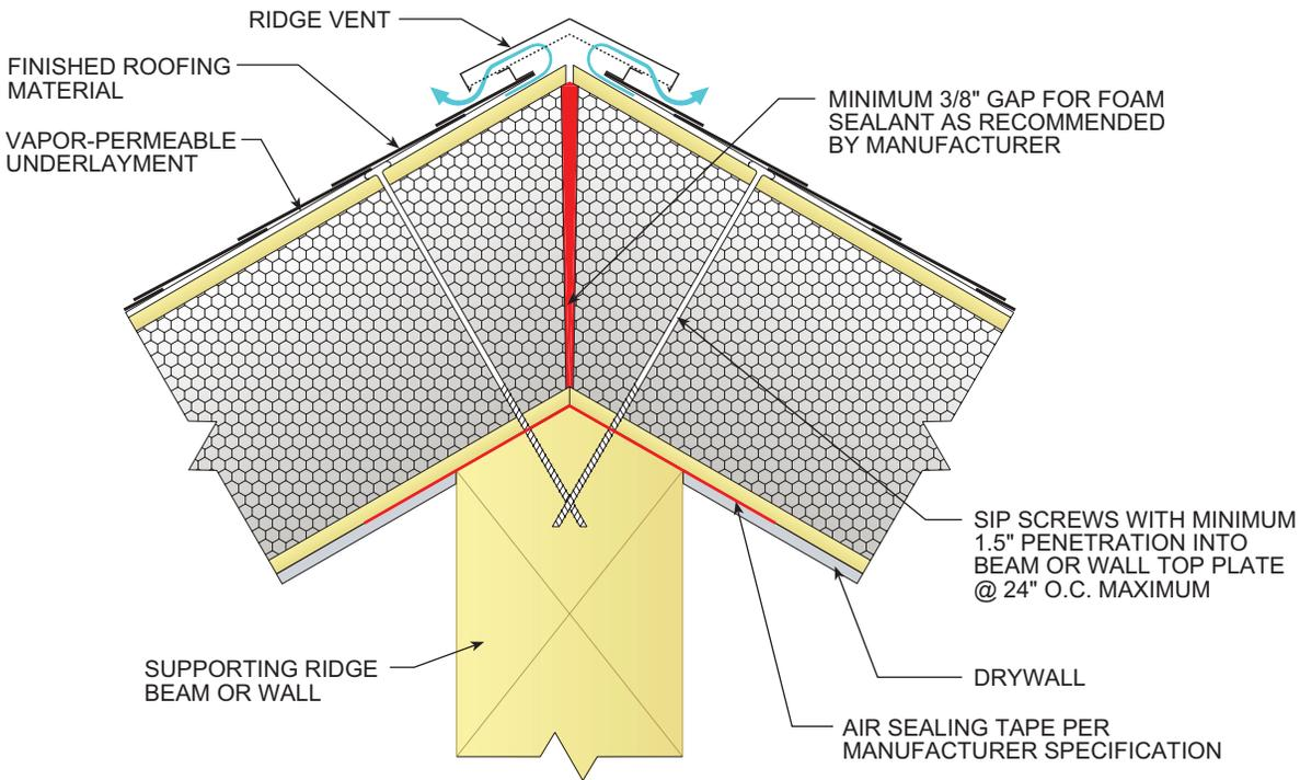
ALL SIP JOINTS SHALL BE AIR SEALED WITH SEALANT AND/OR SIP TAPE. FOLLOW SIP MANUFACTURER'S RECOMMENDATIONS FOR SIP TAPE WIDTHS AND SEALANT PATTERN AND THICKNESSES.
